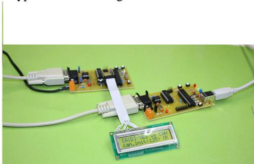
Figure 4: CAN module prototype
