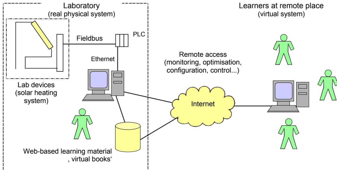
**Figure 1: Real and remote virtual system**
